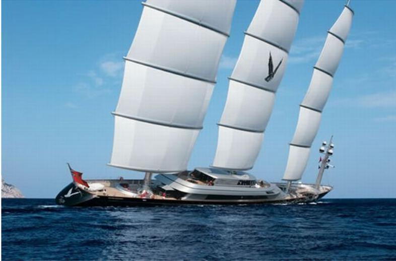
Maltese Falcon, the world's largest sailing yacht 88 meter (289 ft) has been sold for USD 100 million and is built by the Italian Perini Navi Yacht. This boat uses the innovative sailing system DynaRig. It consists of three constantly rotating masts, which hold 15 sails. The maximum speed of the boat is of about 21 knots. Maltese Falcon is able to cross the Atlantic in just 10 days.
