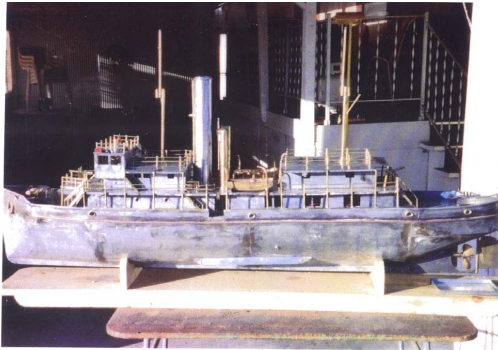
USS San Pablo - Under construction Powered by single 19.2 Volt Motor Driving 3" - Four Blade Pro
